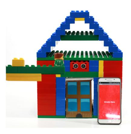
When ultrasonic sensor located nearby window detects intrusion, 'Intrusion Alarm' app rings alarm and send text to family member.
