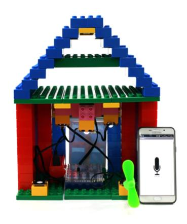
After pressing mic and telling 'turn the light on', 'how is temperature', and 'turn the fan on', the voice recognition remote controller recognizes the order and process the request.
