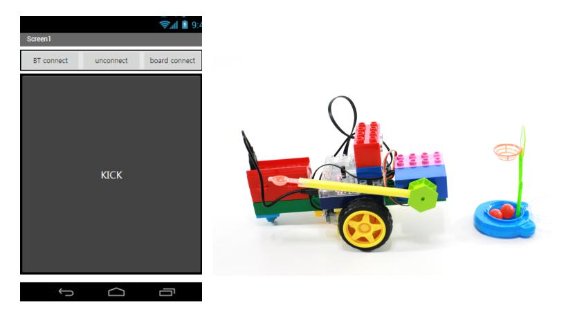
COBL bot can be controlled with built-in gyro-sensor in smartphone by just controlling tilting your phone. When pressing 'KICK' button on screen, the bot can kick a ball.
